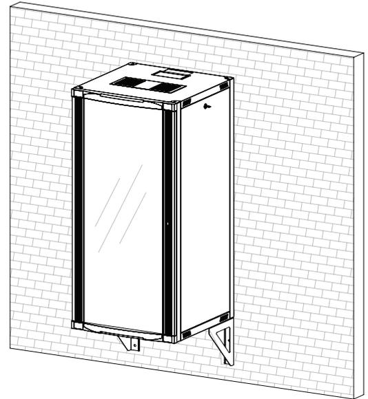
ISOMETRIC VIEW WITH WALL SUPPORT BRACKETS
