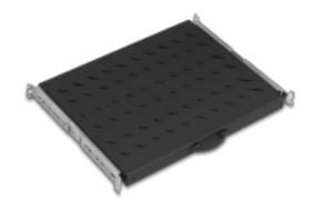
Sliding Shelves, 4 point fixing, Compatible with all brand cabinets Multivendor. Adjustable brackets at depth. For allowing the convection of heated air inside cabinets, the shelves are structured with ventilation slots. Supply is in RAL 9005 Black and RAL 7035 Light Grey colors. From Steel Material, with high technology bending strengthening accessory, Load capacity 50 kg
