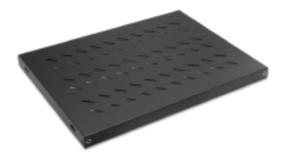
Fixed Shelves, 4 point fixing. For allowing the convection of heated air inside cabinets, the shelves are structured with ventilation slots. Supply is in RAL 9005 Black and RAL 7035 Light Grey colors. From Steel Material, with high technology bending strengthening accessory, Load capacity 50 kg
