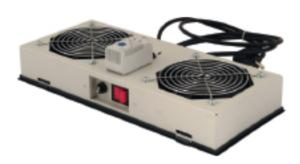
Fan Modules for wall Mounting, Ready pre-installed, plug-in and run style , with on/off switches or with analog thermostat and plugs. Each Fan has an air flow capacity of 2,3-3 cbm/min. Fan Technical data: 18/17 W, 220/240 VAC, 50/60 Hz, 013/0,11 A,2300/3000 rpm 42 dB noise level, Fan life: 10.000 hours
